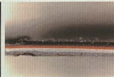
Fig. A29 Paint stratigraphy from door casing in first floor hall (substrate at bottom of photo)
