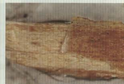
Fig. A20 top right Sample paint stratigraphy for roof elements (substrate at bottom followed by subsequent layers of paint taken from door hinge)
